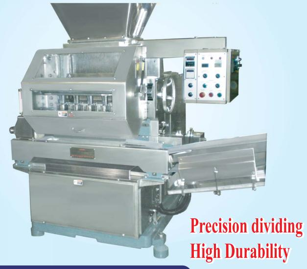
Variation mechanism of dough suction amount in the dough chamber to get high precision dividing.
